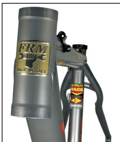
Externally double-butted head tube
