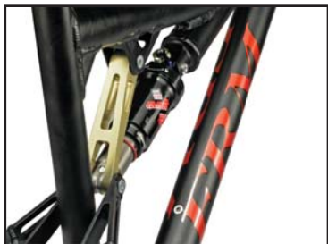
All suspension pivot points rotate on sealed roller and ball bearings
