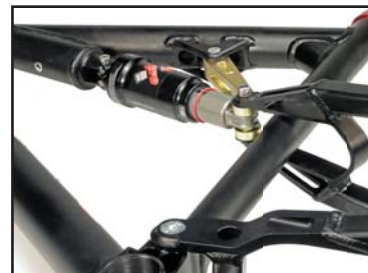
All suspension components are CNC machined from solid billets
