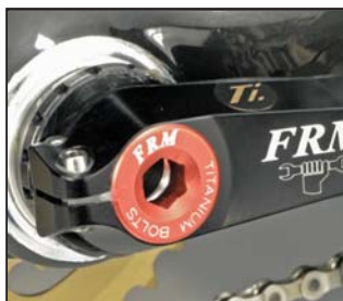
Red Adjusting Plug with Titanium bolts
